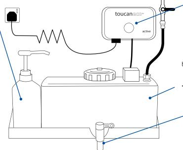
Generator: on/off switch is on the right-hand side. Press button on the front to start activation process, the green light will turn blue for 15 minutes whilst activation process is taking place in the tank. When blue light turns back to green then the solution is ready to use.
